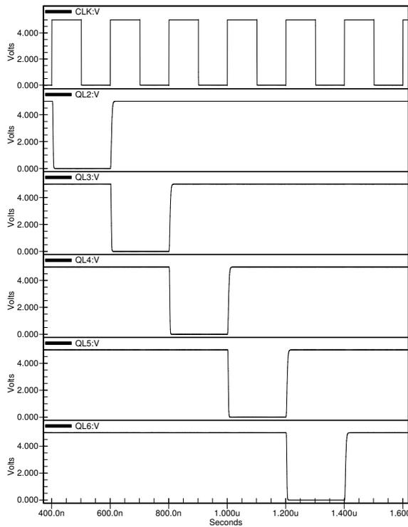
Fig. 8. Functionality of flip-flop at 5Mhz, showing maximum clock rate.
