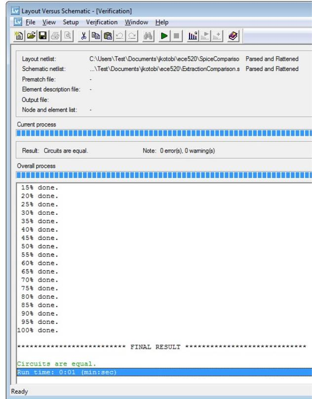
Fig. 9. LVS screen capture showing that the transistor layout is the same as the spice file
