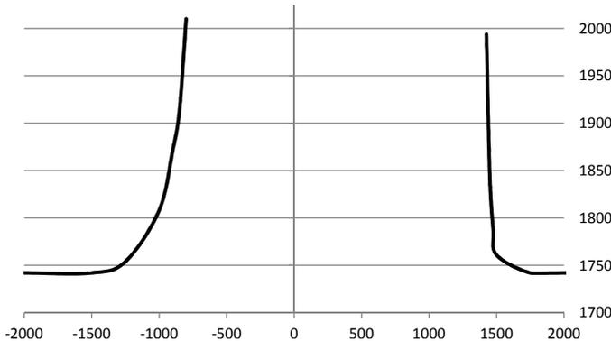
Fig. 3. Setup and Hold Times with extracted transistor capacitance. Axis are picoseconds
