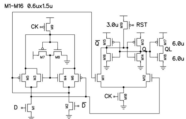
Fig. 2. Transistor Schematic of flip-flop.
