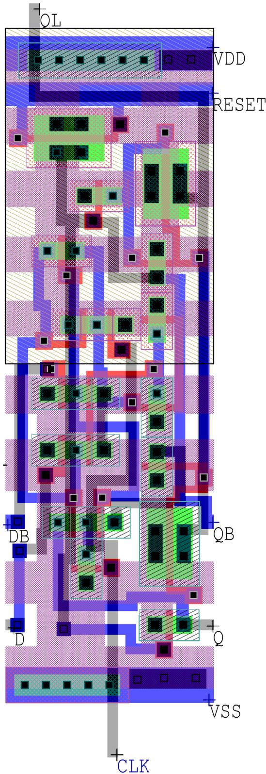
Fig. 5. Flip-Flop Layout used in LVS and DRC checks. 19 transistors total with sizing of  $0.6\mu\text{m}$  and  $2.4\mu\text{m}$
