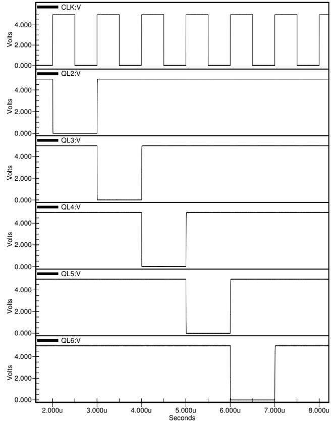
Fig. 4. Functionality of flip-flop at 1Mhz, showing standard operation with a load capacitor of 1.3pF.
